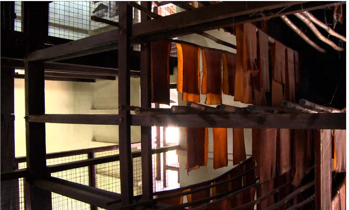
Racks of smoking room for rubber sheets, hung on bamboo poles
